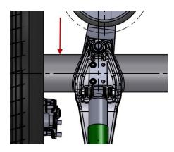
2-The Valx plug has to be removed from the axle spindle and needs to be replaced by a special designed PSI plug for the Valx axle beam.
